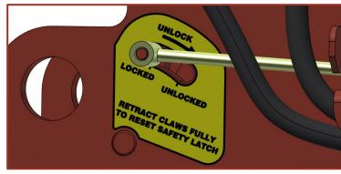
8. Supporting the stowage frame arm using the handles, remove the safety pin **J** and fit into safety pin hole **D** and secure with lynch pin.
