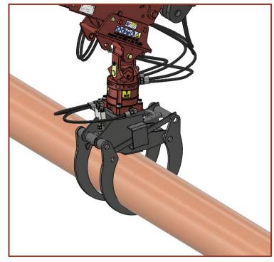
3. Gently lift the crane to ensure the pole has been grabbed in the centre of gravity and is balanced when lifted.
