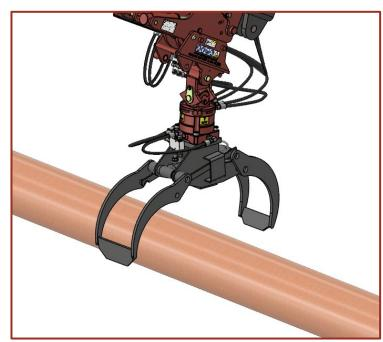
2. Lower the grab to be just above the pole and operate the jaws to tightly close around the pole. The crane may have to be raised or lowered as the jaws close.
