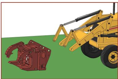
4. Drive the donor vehicle up to the pole grab and position the front forks and so that they align with the holes on the pole grab.
