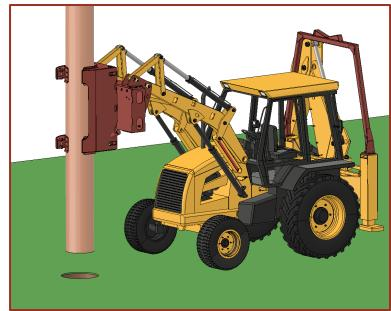
8. Lower the pole into the hole until it touches the bottom by lowering the front forks of the donor machine.
